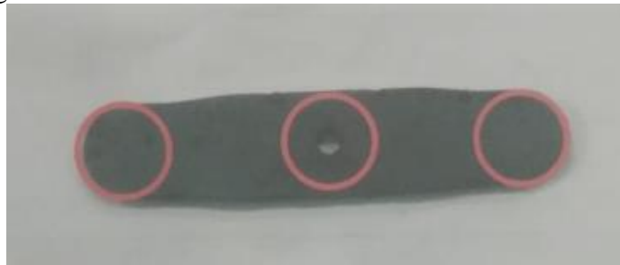
Gambar 9 Hasil Proses Blanking Pierching
