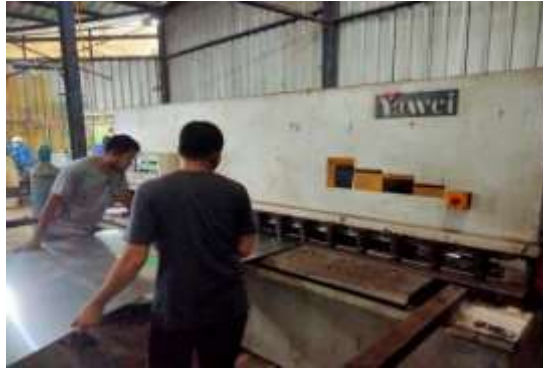
Gambar 2. Cutting Stainless Steel 316L
