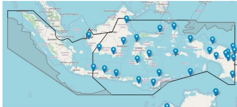
Figure 4. ADS-B ground station coverage at an altitude of 40,000 feet
