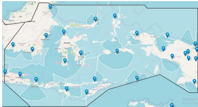
Figure 1. ADS-B ground station coverage at an altitude of 5.000 feet
