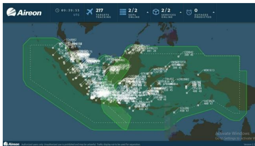
Figure 5. Space based ADS-B ground station coverage at ground zero altitude up to 66.000 feet
