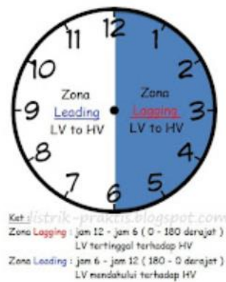
Figure 4. Transformer clock leg and lead zones
