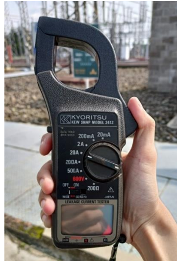
Figure 1 Ampere Clamp Used for Leakage Current Measurement
