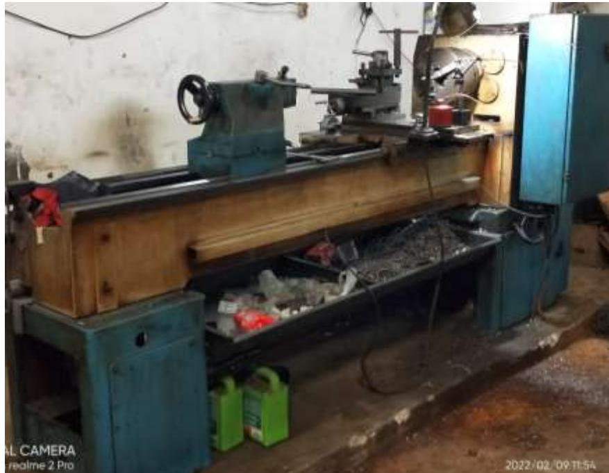
Figure 4. Machined Waste Scattered to the Floor
