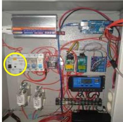
**Gambar 11.** Earth-Leakage Circuit Breaker
