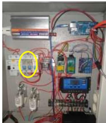
**Gambar 8.** Relay Omron
