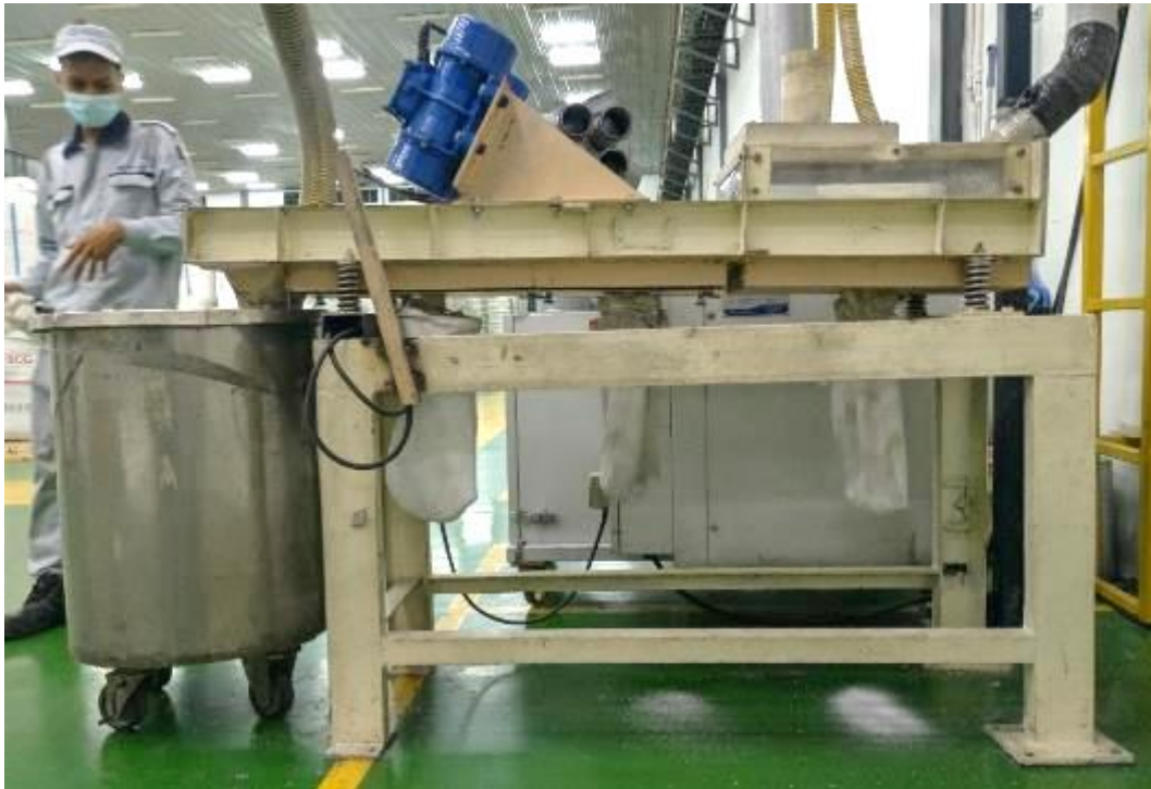
Gambar 8. Tampak Samping Mesin Dust Collector
