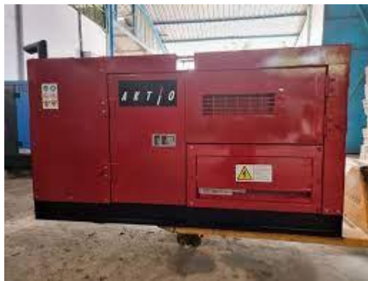
Gambar 1. Genset type silent (Sumber: PT. Aktio Equipment Indonesia)
