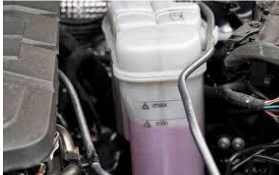
Gambar 4 Level Air Radiator
