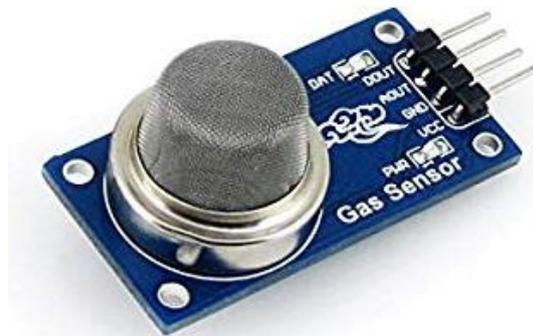
Gambar 2 Sensor Gas MQ-5
