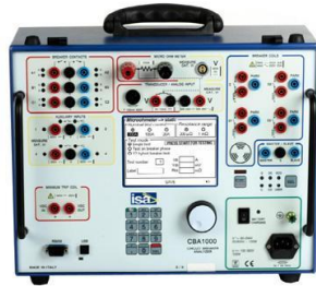
Gambar 2. CBA 1000 – Circuit Breaker Analyzer and Micro-ohmmeter
