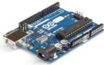
**Gambar 1. Papan Arduino Uno R3**
