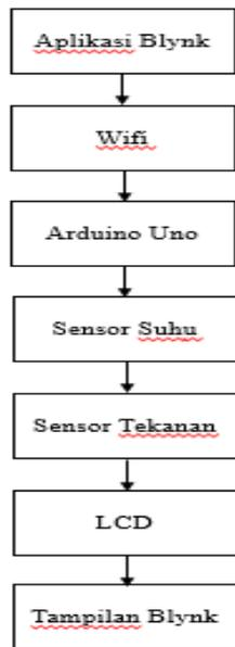
**Gambar 5. Diagram Blok Sistem**
