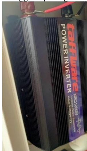
Gambar 17. Inverter 1000W DC 12V to AC 220V
